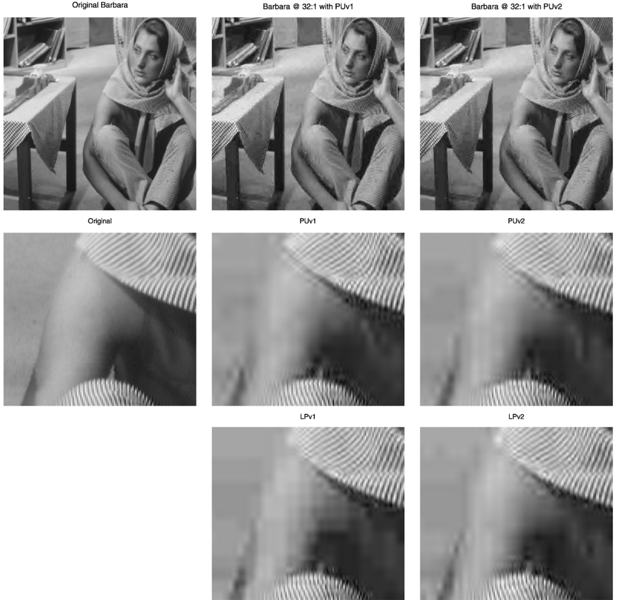
Fig. 8. Compression results at 32:1 for visual comparison. The original image and a zoomed-in patch are shown in the first column. The reconstructed images and their zoomed-in patches using one- and two-regular 8 \times 24 PUFBs are shown in the second and the third columns, respectively. Notably, the current design PUv1 produces a much smoother reconstruction than LPv1.
